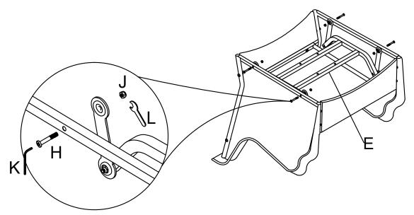
Step 6: Attach swivel base (F) to rocking base (E) with 12 washers (I&M), 4 nuts (J) and 4 screws (H) by using allen wrench (K) and spanner (L). Verify the alignment and adjust and fully tighten all the screws.
