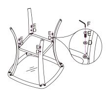
STEP 2: Assemble table tray (C) to 4 table legs (A) by using 4 screws (E) and 4 washers (D) with allen wrench (F). Do not tighten all bolts now.
