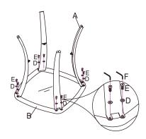
STEP 1: Assemble 4 table legs (A) to glass table top (B) by using 8 screws (E) and 8 washers (D) with allen wrench (F). Do not tighten all screws now.
